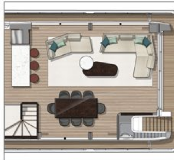
MAIN DECK SALOON SHOWN WITH EXTENDED SOFA SEATING, GALLEY BAR WITH STOOLS AND PORT SIDE DINING
